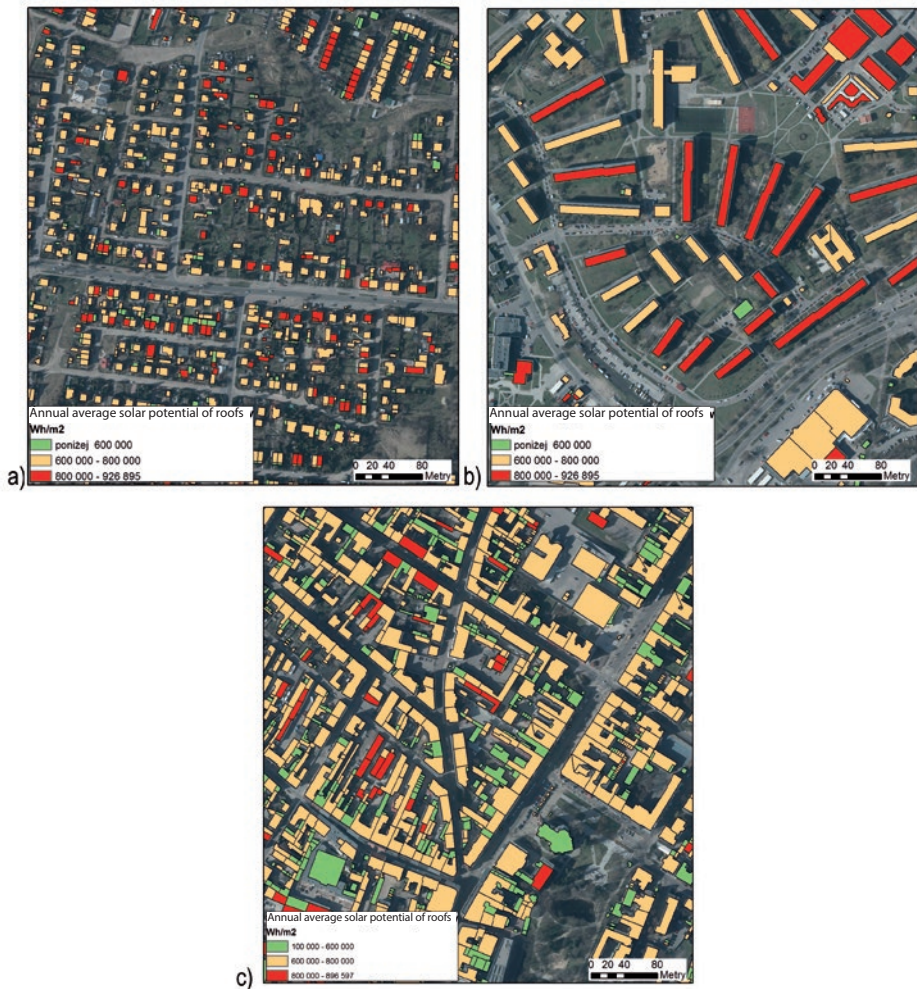
Fig. 7. The solar potential of the roofs of the buildings in Wh/m 2 in Bydgoszcz: a) in single-family houses settlement; b) in multi-family houses settlement; c) in the city centre
