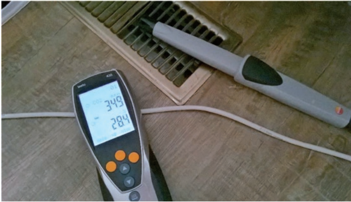
Figure. 1 Measurement of outer concentration CO 2 on outlet (Testo 435-2 and sensor of IAQ)
