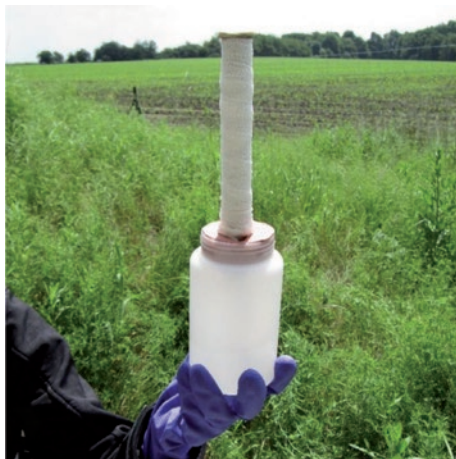
Figure 11: The “wet candle” method for the determination of chloride deposition
