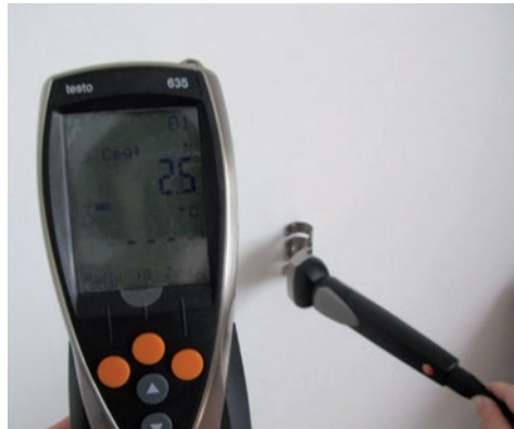
II.3. The humidity of the wall and the heat transfer coefficient for a warmed wall were measured using Multifunction Testo 435-2.
